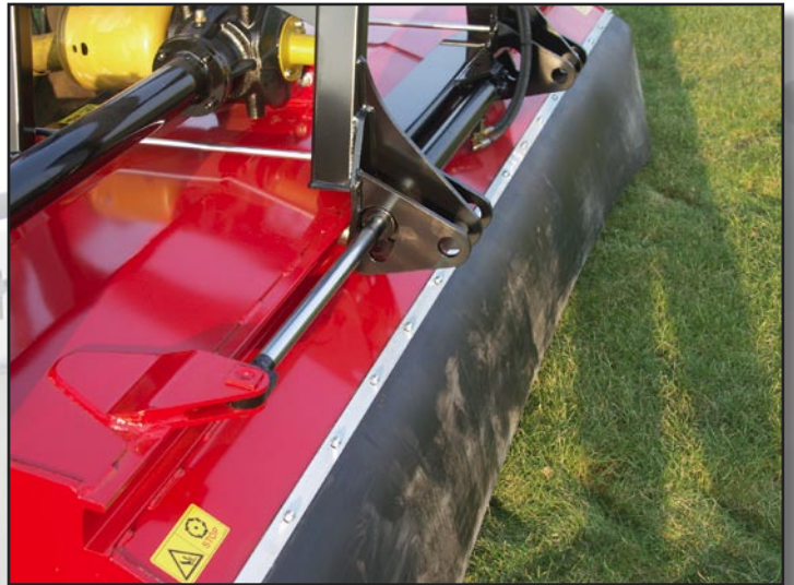
Side shift 60 cm (with double 3-points linkage)
