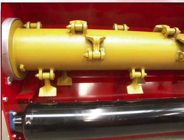
Rotorshaft Ø 245mm
